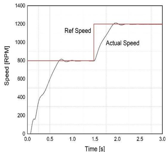
Figure 5. Step response from Standstill
