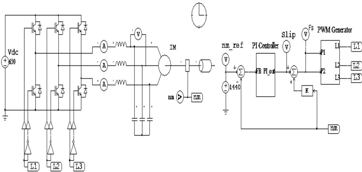
Figure 4. Functional Block implementation for Simulation in PSIM
